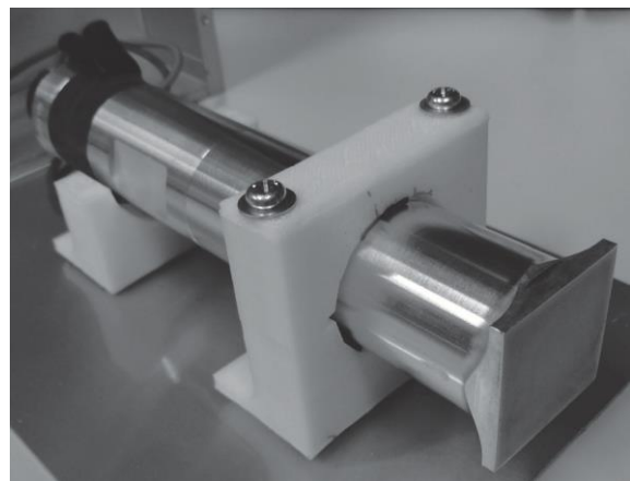
Fig. 3 Langevin type ultrasonic transducer with horn
